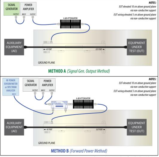
Figure 19 - Examples of Typical Test Setups
