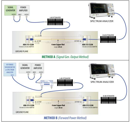
Figure 18 - Example Equipment Arrangements for Test Level Calibration
