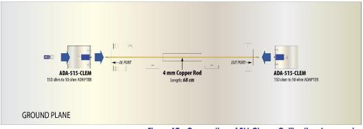
Figure 17 - Connection of EM Clamp Calibration Accessories
