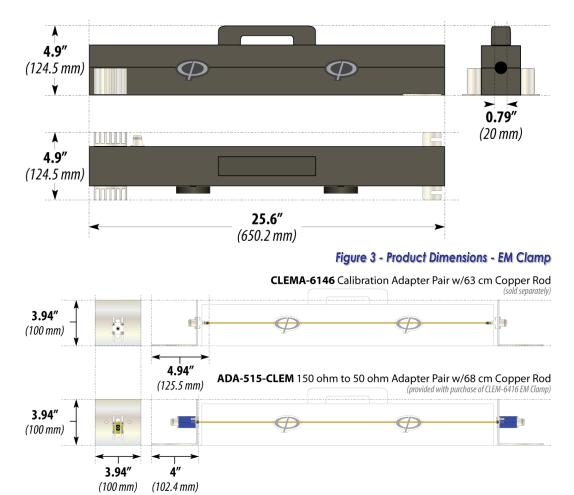
Figure 4 - Product Dimensions - EM Clamp Adapters and Accessories
