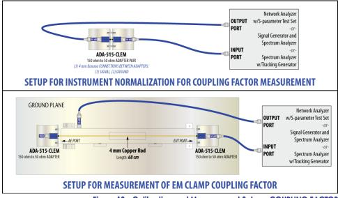
Figure 12 - Calibration and Measurement Setup - COUPLING FACTOR
