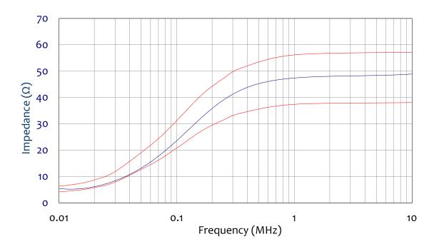
Figure 6: Typical Impedance compared to Mil-Std requirements
