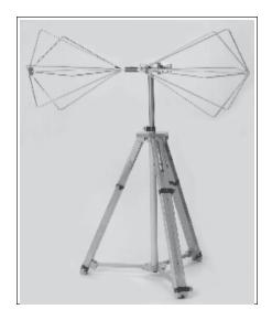
Figure 1.1 Biconical Antenna (w/ tripod AT-100)
