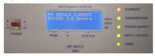
8. In order to restart the unit, first turn off the front panel switch, and then restart the unit as described in Section 3.
