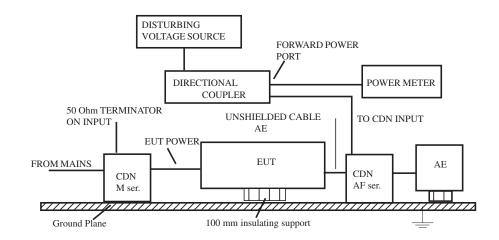
Figure 3-1 Conduted Immunity test setup using S series CDNs
